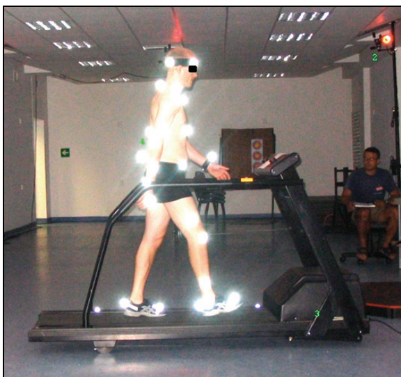
Fig. 1. The manner of carrying out the study: 1, 2 – cameras, 3 – treadmill, 4 – subject during registration session (photo: G. Latocha)
