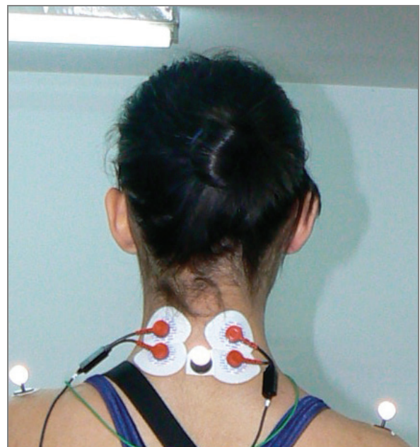
Fig. 1. Electrode location during measurement
