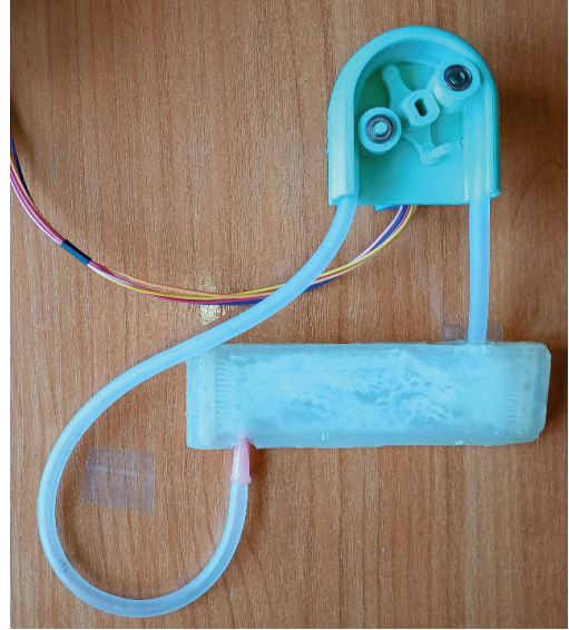
Fig. 8. The peristaltic micropump connected to specimen
