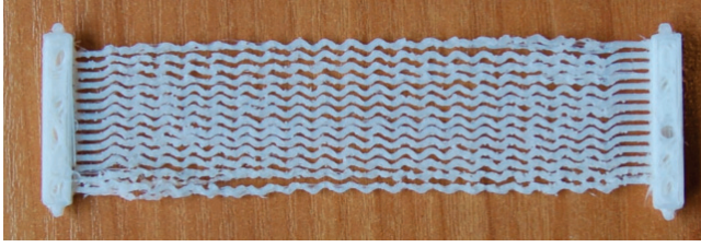
Fig. 6. Fiber arrangement in the inner layer of the material sample with fixing elements
