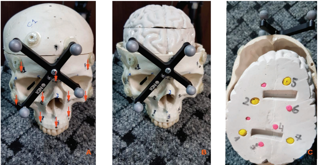
Fig. 1. Skull and brain phantom with 7 tumor lesions in three different configurations: A – skull phantom, arrows indicate fiducials, B – brain, C – target plane with tumor lesions
