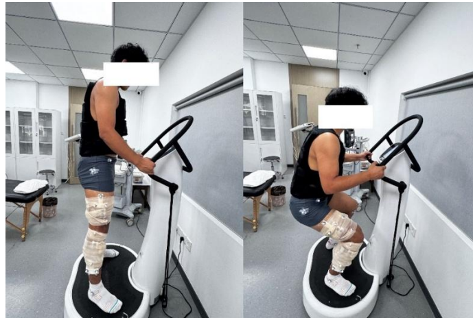
Figure 1. Loaded whole-body vibration (WBV) training setup. participant performing dynamic squats on a vertical vibration platform (20 Hz, 6 mm) while wearing a weighted vest (20% body mass).
