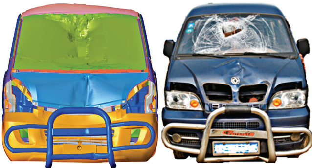
Fig. 7. Deformation traces in the minivan of the simulation
