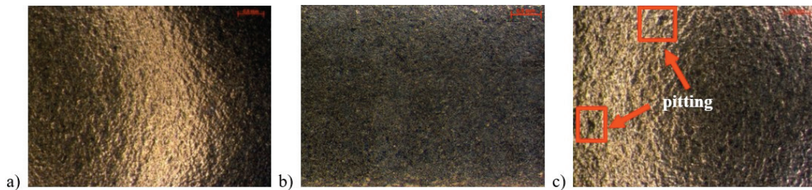
Fig. 17. Examples of corrosion damage on the samples: a) PE, b) PES, c) PESR, mag. 18.9 \times
