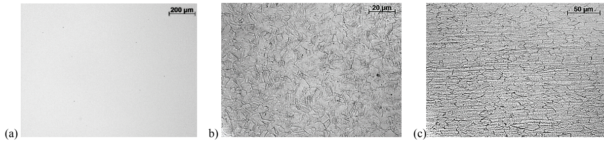
Fig. 3. Non-metallic inclusions in the form of globular oxides: (a) austenitic structure with slip bands transverse, (b) longitudinal, (c) light microscope
