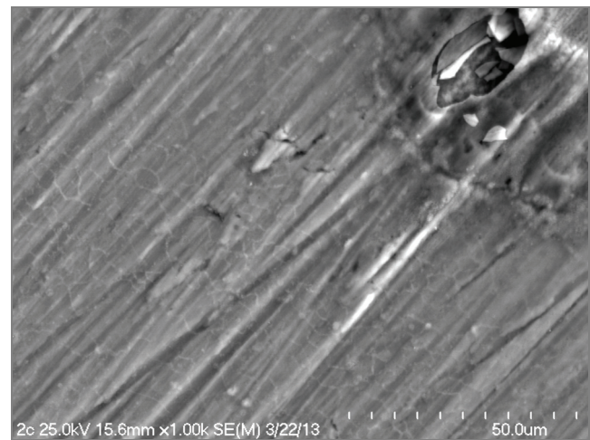
Fig. 7. SEM-SE surface state of profile-milled sample after oxidation and single firing and after potentiodynamic tests
