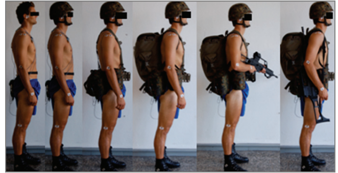
Fig. 1. Location of markers (from left to right) and order in which equipment was added: control, helmet, load-carrying equipment, backpack, rifle (in front of the body) and rifle (slung over the right shoulder)
