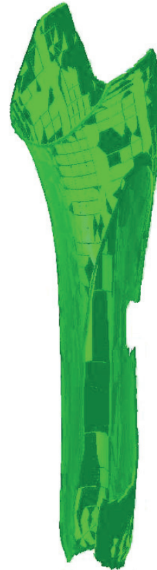
Fig. 5. Contact area: in this case the prosthesis has no proximal contact; distally, it contacts the bone anteriorly; this boundary condition is not recommendable because it is very likely to produce stress shielding
