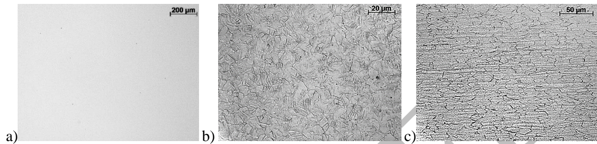
Fig. 3. Non-metallic inclusions in the form of globular oxides – a), austenitic structure with slip bands – transverse b), longitudinal – c), light microscope
