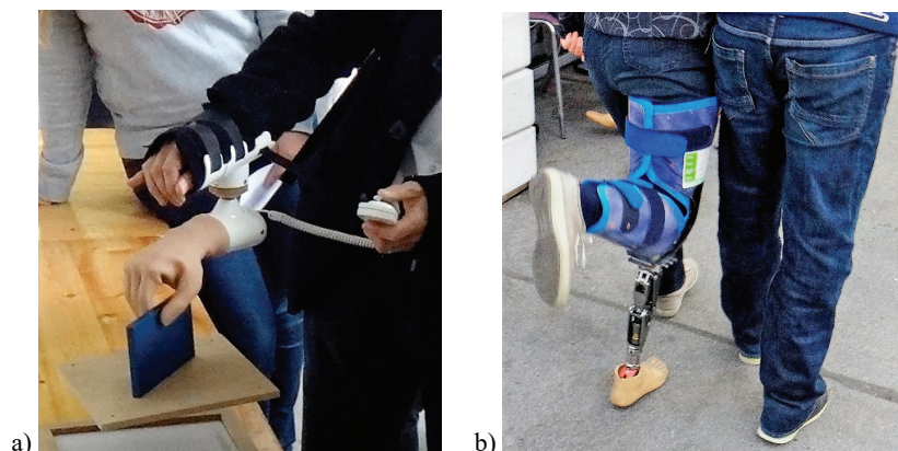
Fig. 4. During „Cybathlon” spectators could try devices for disabled people: a) artificial hand, b) artificial lower leg
