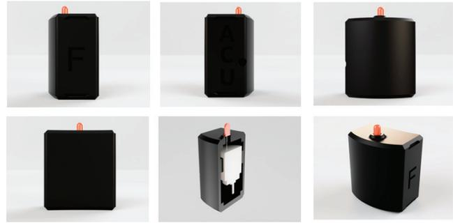
Fig. 1. 3D printed cases (using stereolithography) of the vibration units (Autodesk Fusion 360 TM CAD (<https://www.autodesk.com>) Formlabs Form 2<sup>®</sup> (<https://formlabs.com>))
