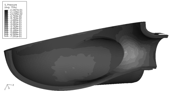
Fig. 7. Distributions of average stress at inner surface of bottom part of chamber (side view of cross-section)
