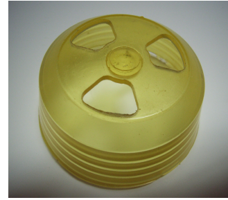
Fig. 2. Photoelastic model of the cup
