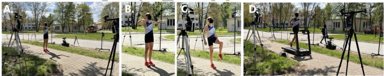
Fig. 1 A) Measurement space; B) Motorcyclist position - standard calibration; C) Dynamic calibration; D) Tests on a mechanical treadmill.
