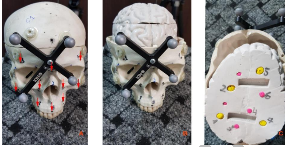
Figure 1. Skull and brain phantom with 7 tumor lesions in three different configurations: A – skull phantom, arrows indicate fiducials, B – brain, C – target plane with tumor lesions.
