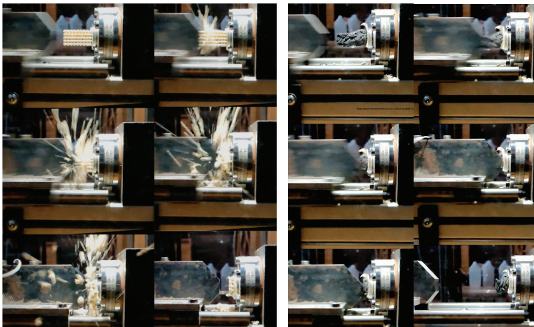
Fig. 4. The courses of destructive tests of a ball sample and an EPS sample cut from the helmet
