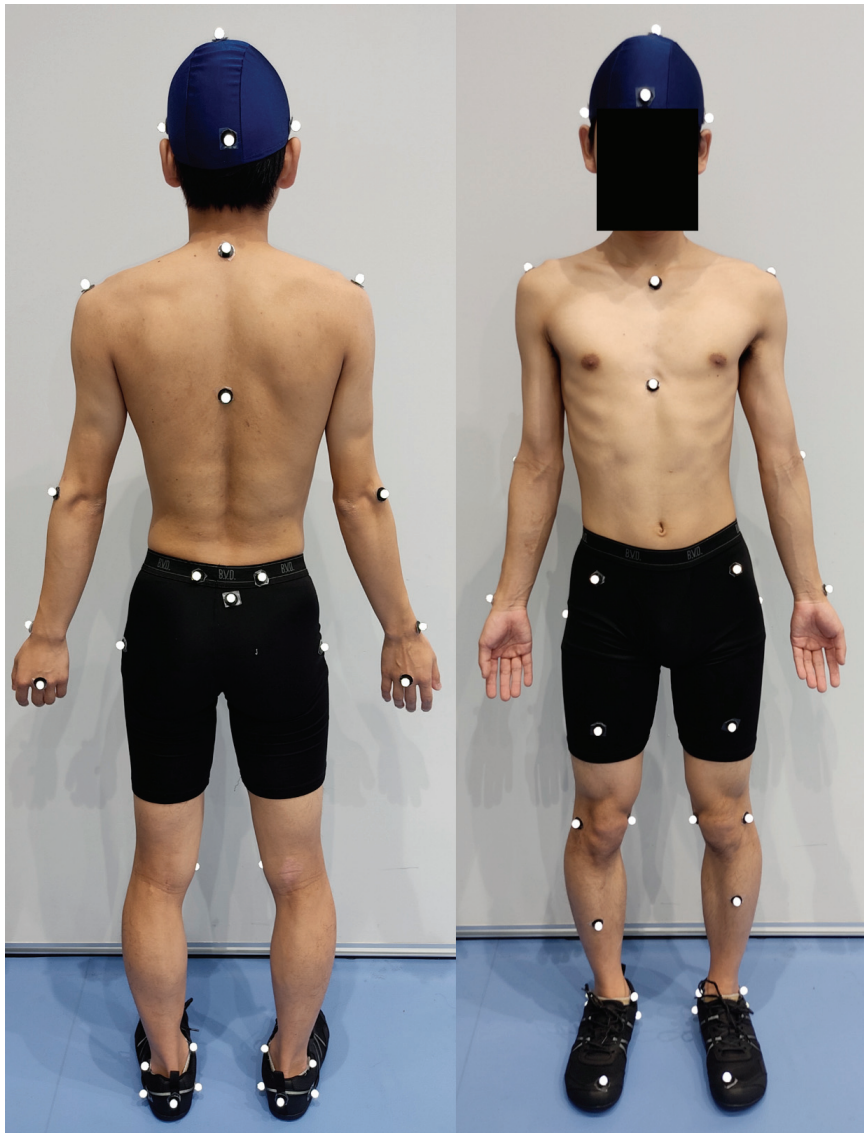
Fig. 2. Placement of reflective markers on the full body
