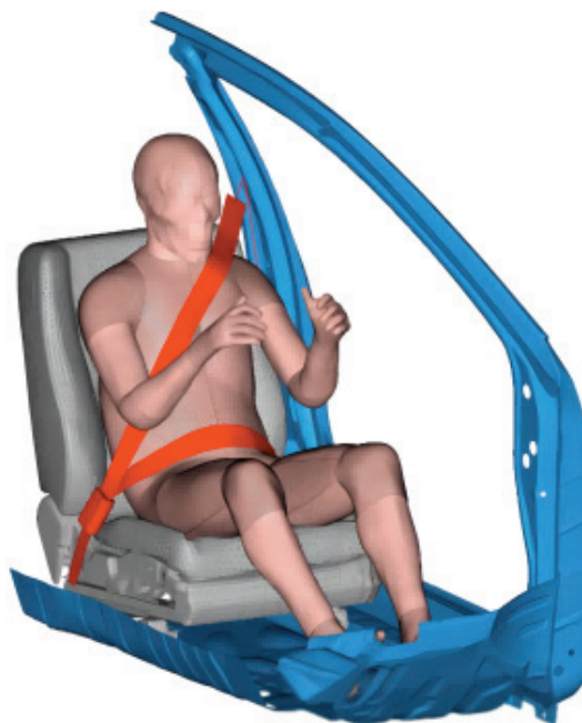
Fig. 1. Vehicle–seat–occupant subsystem FE model
