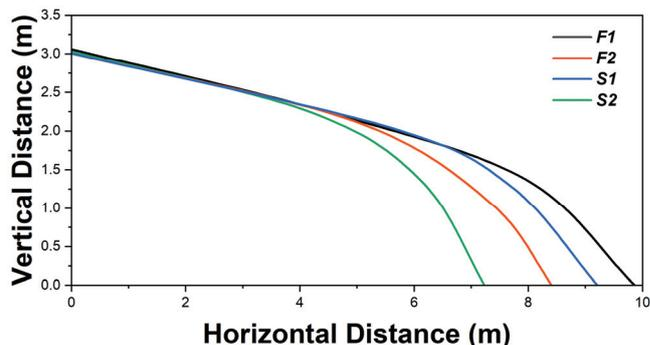
Fig. 8. Simulated trajectories for four shuttlecock models on a smash shot
