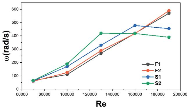
Fig. 4. Rotation rate vs. Reynolds number for four shuttlecock models
