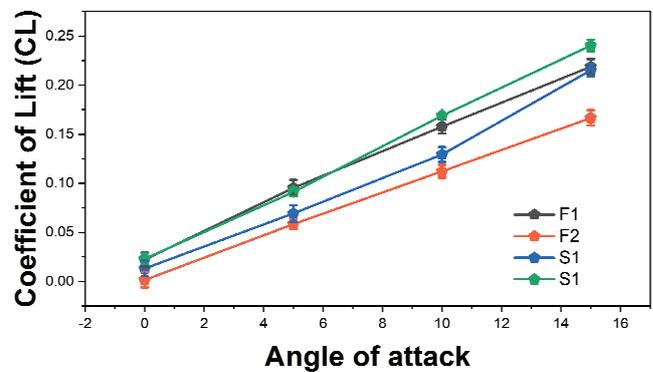
Fig. 3. Lift coefficient vs. angle of attack at  $Re = 2 \times 10^5$  for four shuttlecock models
