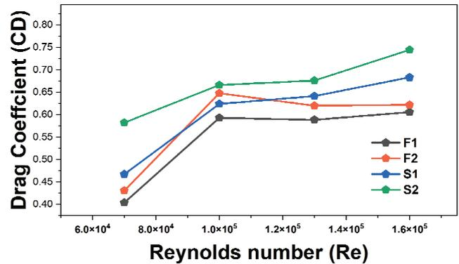
Fig. 2. Drag coefficient vs. Reynolds number at  $\alpha = 0^\circ$  for four shuttlecock models
