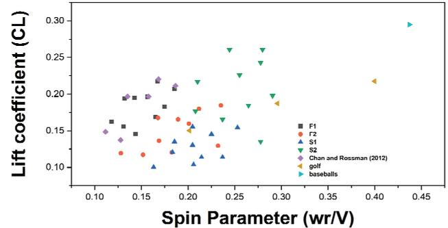
Fig. 5. Lift coefficient vs. spin parameter for four shuttlecock models
