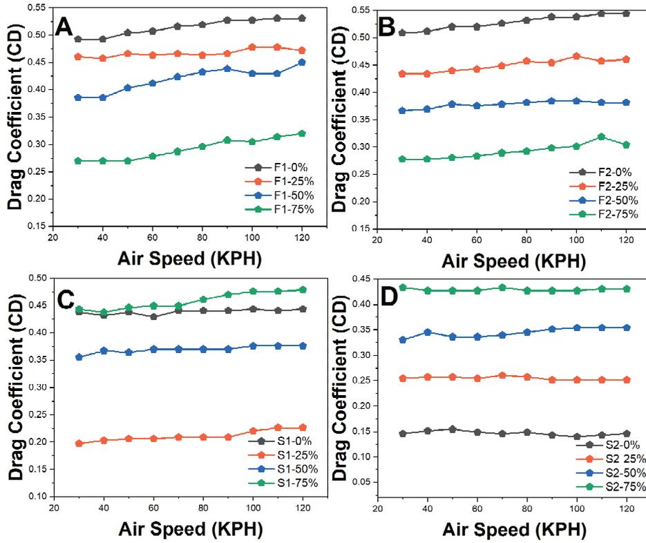
Fig. 6. Drag coefficient vs. gap porosity at  $Re = 2 \times 10^5$ ,  $\alpha = 0^\circ$  for four shuttlecock models
