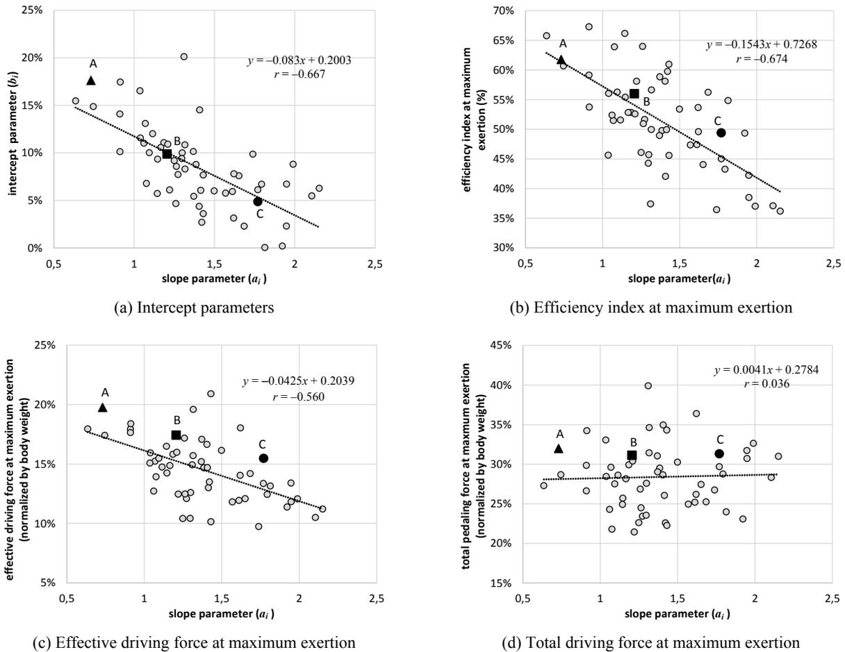
Fig. 4. Relationship between slope parameters and other measured values: (a) intercept parameters, (b) efficiency index at maximum exertion, (c) effective driving force at maximum exertion, and (d) total driving force at maximum exertion
