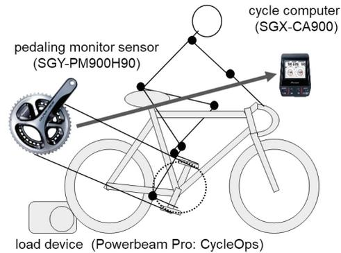
Fig. 1. Overall structure of the data recording system
