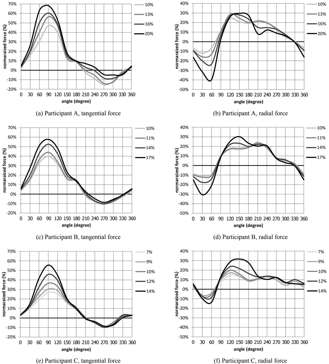
Fig. 5. Typical tangential and radial force normalized by body weight due to crank angle changes as the average force exerted increases (Participants A, B, and C)
