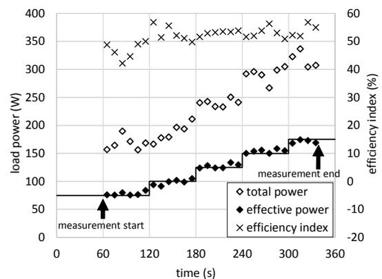
Fig. 2. Experimental protocol and example of measurement
