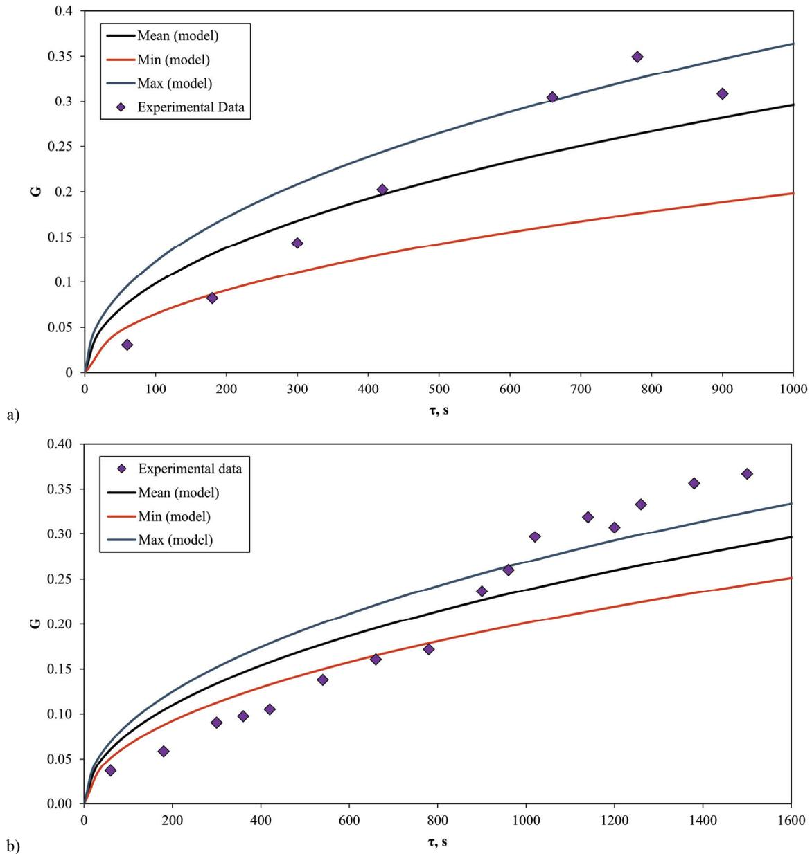
Fig. 5. Experimentally determined conversion in time and GB model using minimum, average and maximum values for a kinetic constant for: (a) 0.15 M  $\text{Ca}(\text{OH})_2$  suspension, (b) 0.30 M  $\text{Ca}(\text{OH})_2$  suspension
