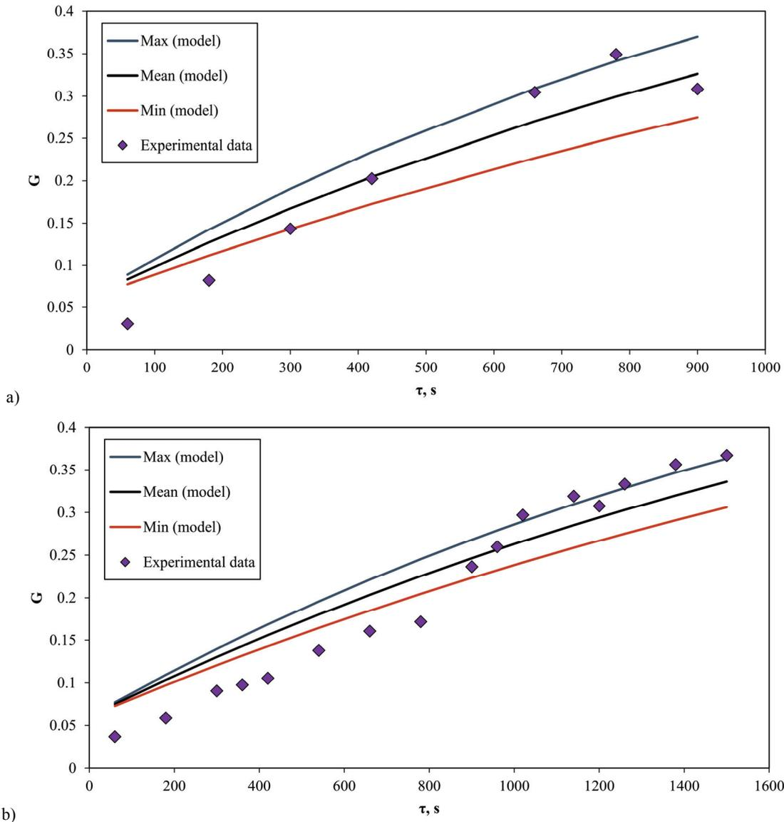
Fig. 6. Conversion evolution in time obtained using regression analysis of experimental data of: (a) 0.15 M  $\text{Ca(OH)}_2$  suspension and (b) 0.30 M  $\text{Ca(OH)}_2$  suspension series
