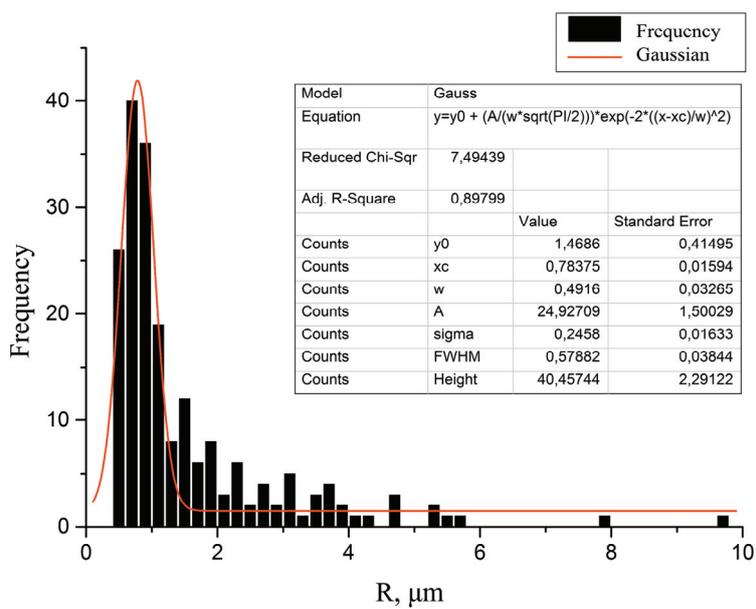
Fig. 3. Particle size distribution
