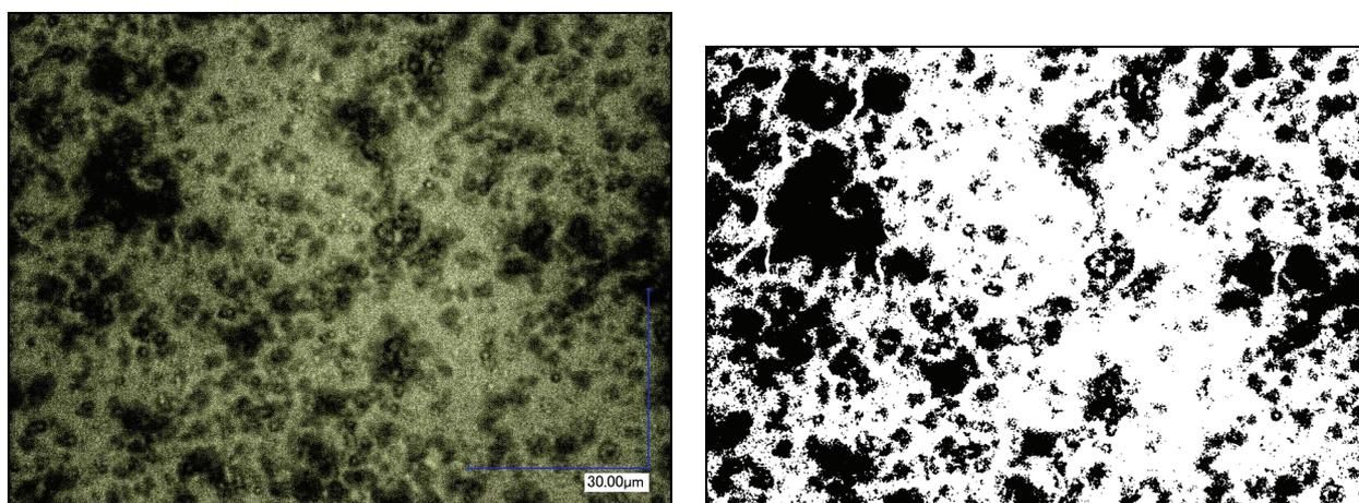
Fig. 2. Calcium hydroxide suspension after the ball mill; left: view in a digital microscope; right: after noise removal as used for particle size analysis (particles used for analysis are marked in black)
