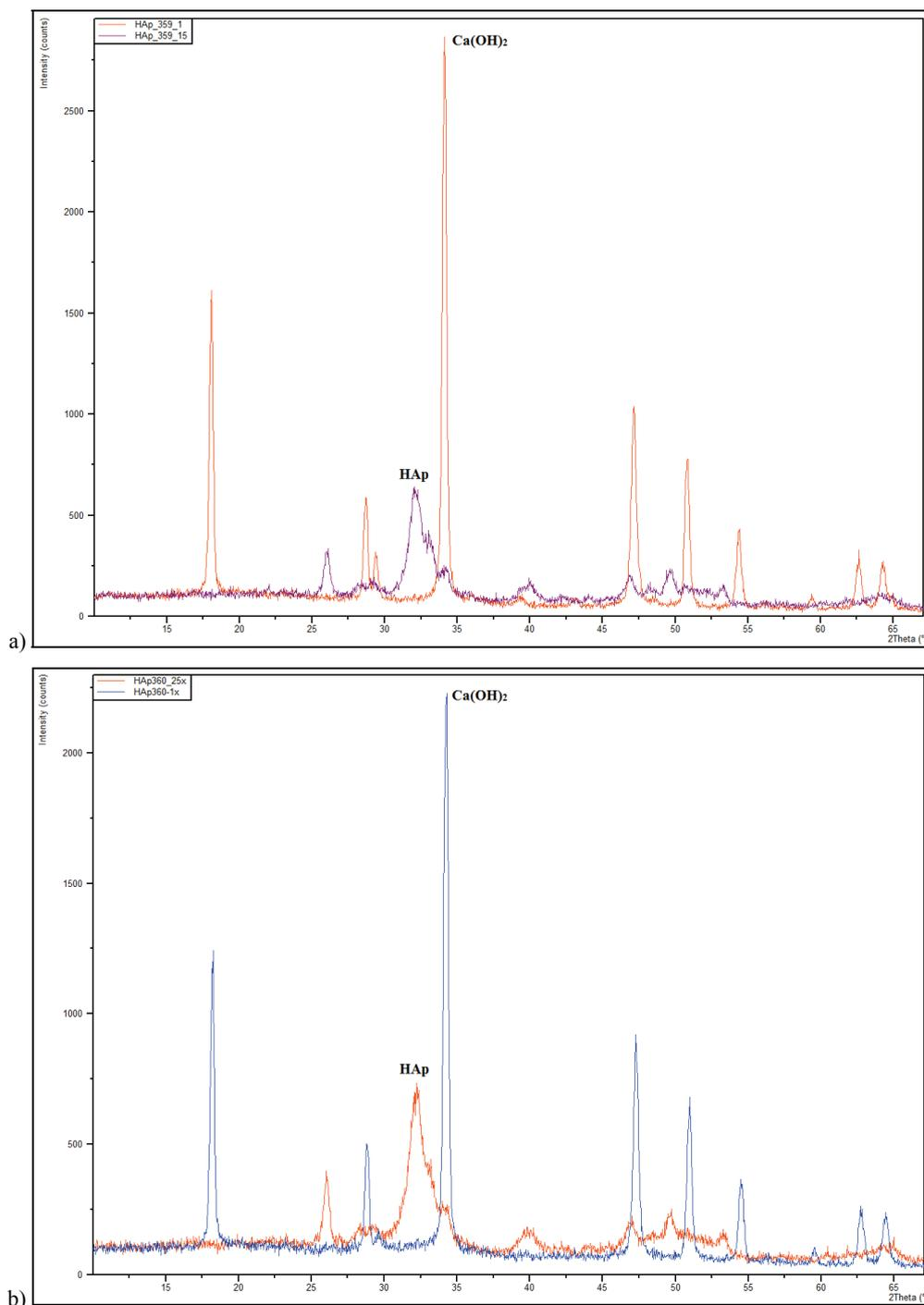
Fig. 4. First and last diffractograms of (a) 0.15 M  $\text{Ca}(\text{OH})_2$  suspension and (b) 0.30 M  $\text{Ca}(\text{OH})_2$  suspension
