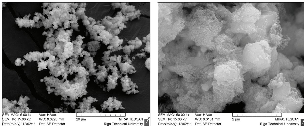
Fig. 1. SEM micrographs of Ca(OH)<sub>2</sub> used for particle size determination
