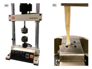
Fig. 1. Uniaxial testing machine MTS 858 MiniBionix<sup>®</sup> (a) and the specimen between grips during the test (b)
