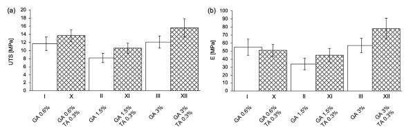
Fig. 4. Increase in (a) UTS values by 17% to 29% and (b) *E* values by 32% (series XI) and 37% (XII) noted after TA additional cross-linking
