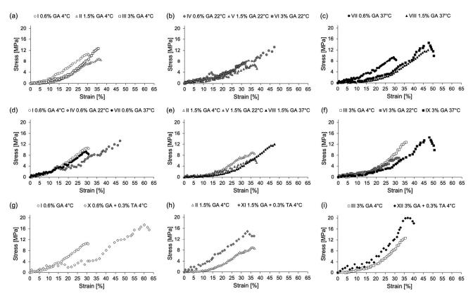
Fig. 3. The stress–strain curves for specimens cross-linked in: (a) 4 °C; (b) 22 °C; (c) 37 °C; (d) 0.6% GA; (e) 1.5% GA; (f) 3% GA; (g) 0.6% GA + 0.3% TA; (h) 1.5% GA + 0.3% TA; (i) 3% GA + 0.3% TA
