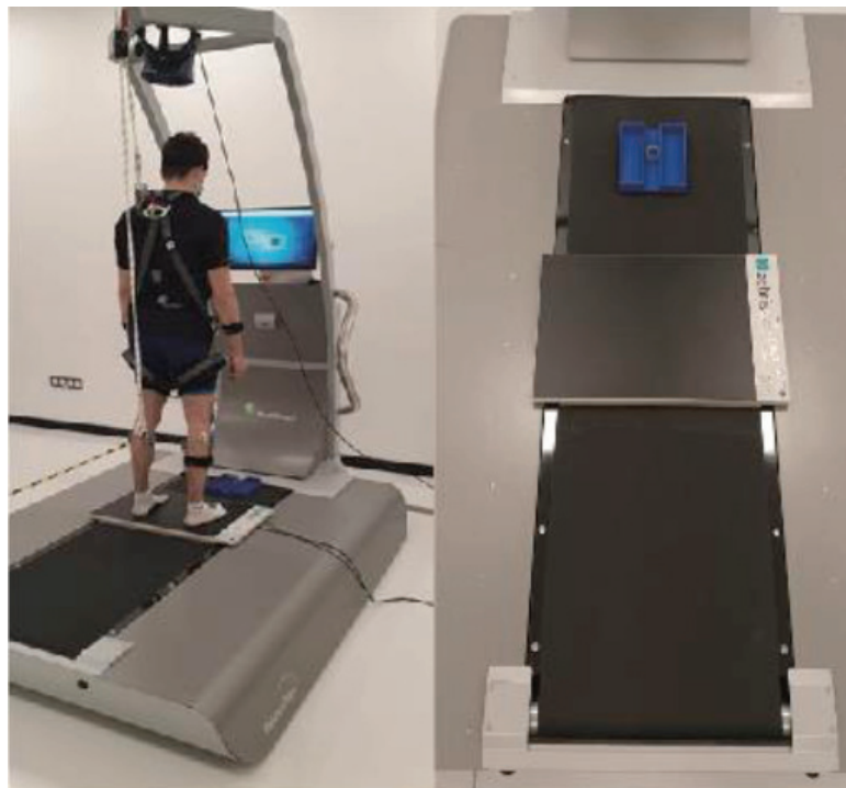
Fig. 1. Measurement stand with a test participant and the treadmill with the sensor and direction of perturbation
