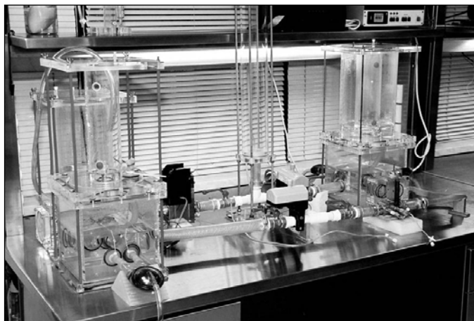
Fig. 1. Mock circulation with Ventricular Assist Devices POLVAD-MEV designed by Z. Nawrat at the Institute of Heart Prostheses in Cardiac Surgery Development Foundation in Zabrze
