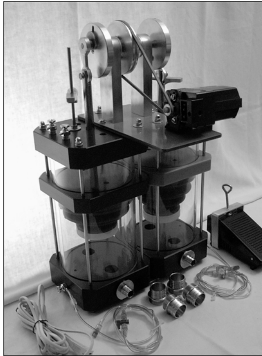
Fig. 2. Physical model of inlet and outlet compliance designed and made by M. Paszkowski based on Windkessel's theory
