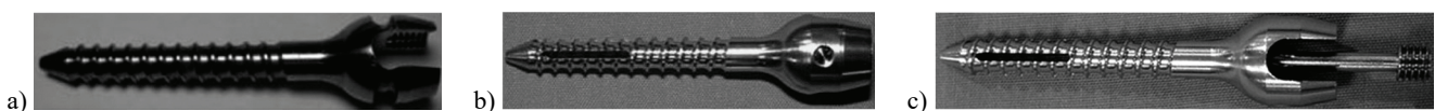
Fig. 1. Usage of the pedicle screws in this study including conventional solid pedicle screws (a), cannulated pedicle screws (b), and cannulated pedicle screws with a central pin (c)
