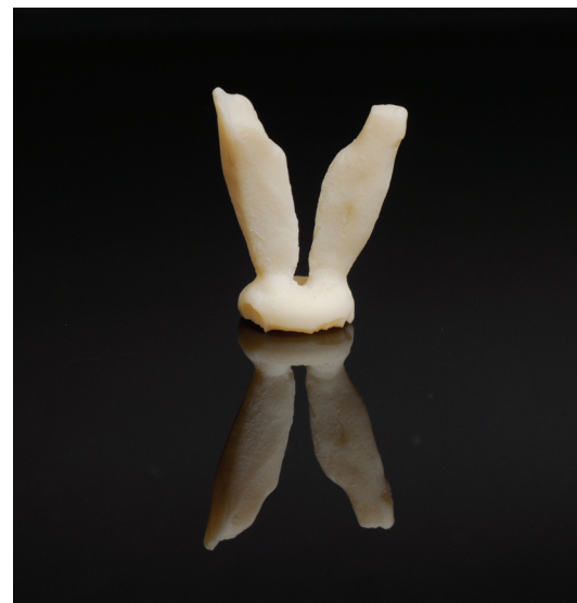
Fig. 2. Ceramic phantom before being embedded in acrylic base
