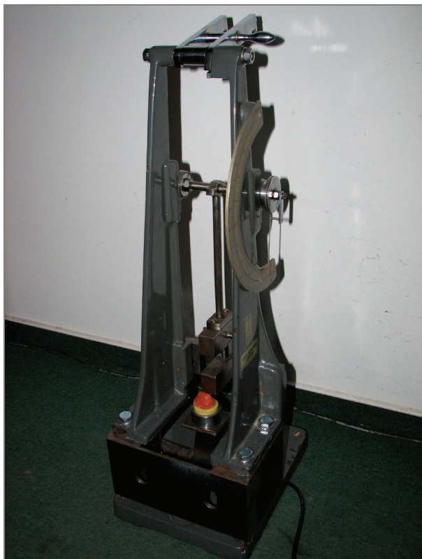
Fig. 4. Polymer sample placed on the ceramic phantom, which was set in the support stand of the Charpy hammer
