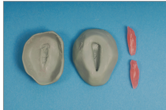
Fig. 1. Silicone form and wax models of ceramic phantom
