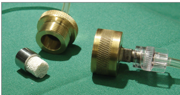
Fig. 1. The central part of our experimental setup, showing the hydroxyapatite scaffolding, with its stainless steel tube and the brass holder used when applying fluid pressure
