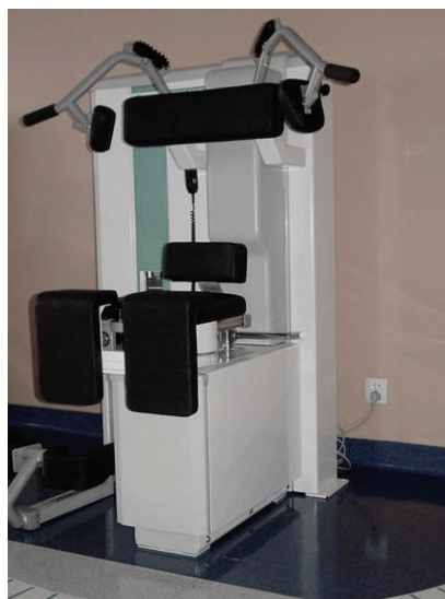
Fig. 3. LTR – DBC device for diagnostics and active resistance exercise of lumbar thoracic spine rotation
