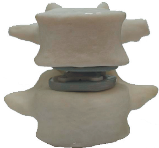
Fig. 6. 3DP model of L4-L5 spinal motion segment with the INOP/LSP.1101 endoprosthesis placed in the intervertebral space
