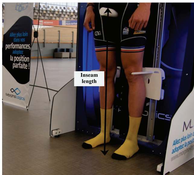
Fig. 1. Inseam length measurement with the ML Size ®
