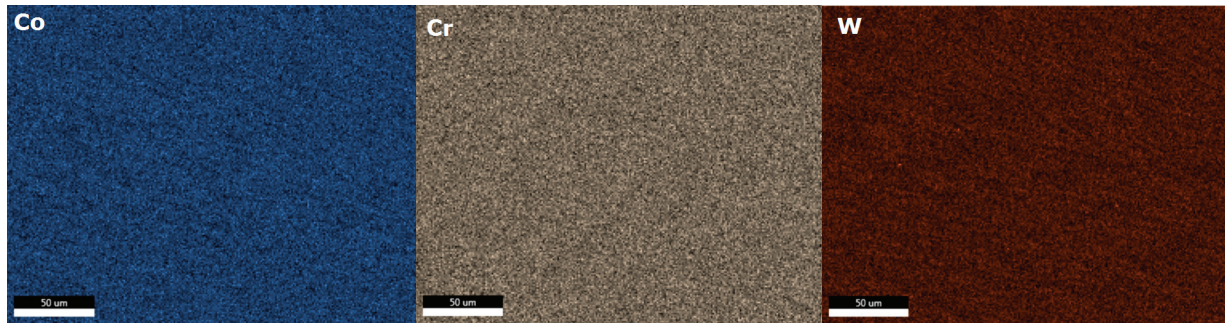
Fig. 4. EDS maps of elemental composition for cobalt (Co), chromium (Cr) and tungsten (W)
