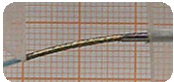
Fig. 10. Crimped stent during one-point bending test
