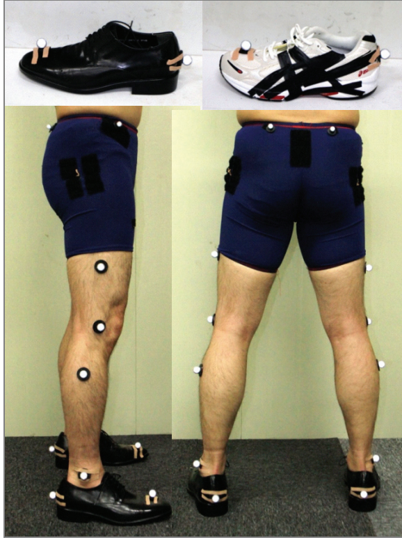
Fig. 1. Testing shoes and marker locations: dress shoe (top-left) and running shoe (top-right) with retro-reflective markers (toe and heel), and locations of sixteen body markers from sagittal view (bottom-left) and back view (bottom-right)
