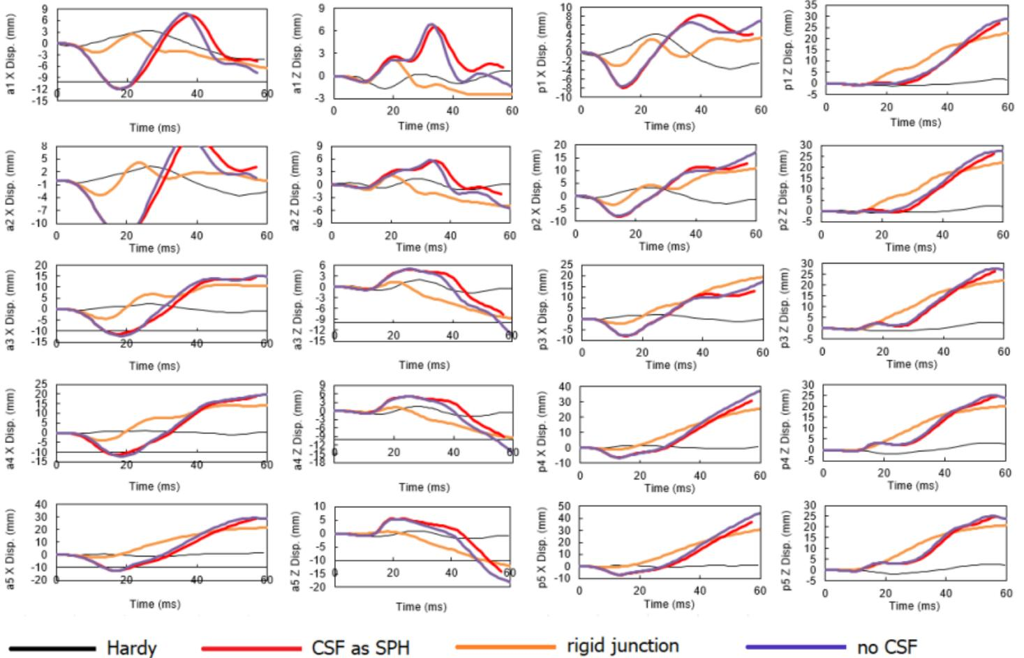
Figure 8. Benchmark aHEAD simulation (CSF as SPH) with two modified head models: “rigid junction” and “no CSF”. The displacements are compared with Hardy C755-T2 test results.
