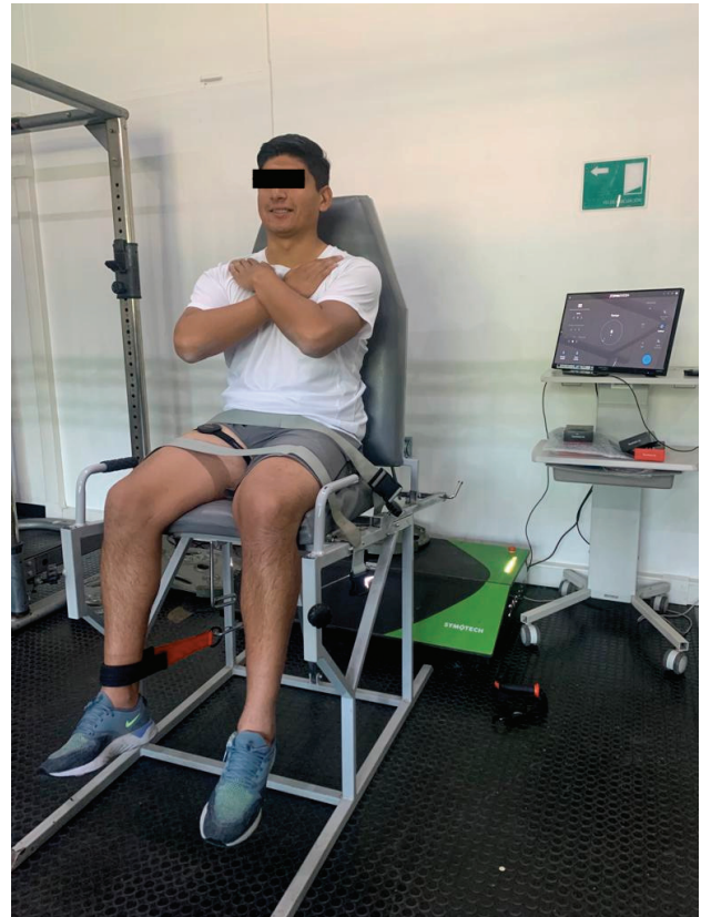
Fig. 1. Evaluation of muscle strength P1, P2 and P3 and fixation of the dynamometer at the distal end of the leg to provide resistance to each protocol
