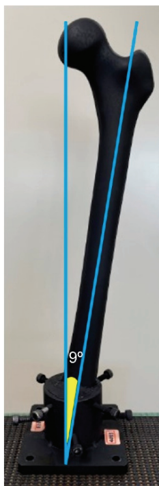
Fig. 2. Image of the setting of a synthetic femur
