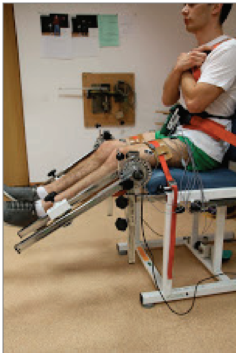
Fig. 2. Measurement of PT and EMG signal in flexors of the calf in the knee joint
