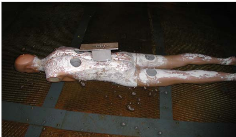
Fig. 5. The previously balanced mannequin immersed in the hydraulic flume
