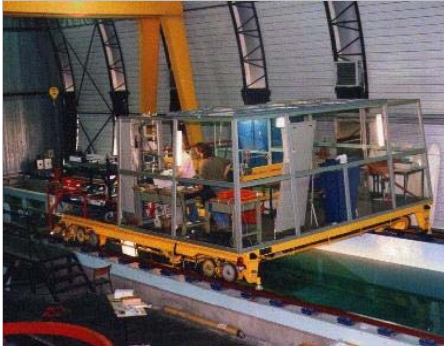
Fig. 2. The mobile carriage in the hydraulic flume. The mannequin has been fixed below the carriage and then 50 m carried on
