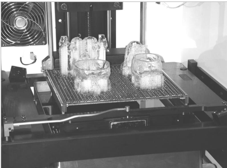
Fig. 5. The medical models manufacturing with SLA-250, Rzeszów University of Technology
