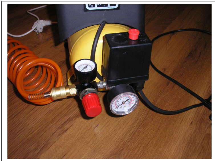
Fig. 3. Compressor with reducer and pressure switch
