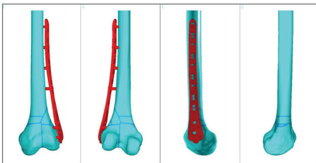
Fig. 4. LISS locking plate mounted on a model of the femur. Anterior, posterior, lateral, and medial views
