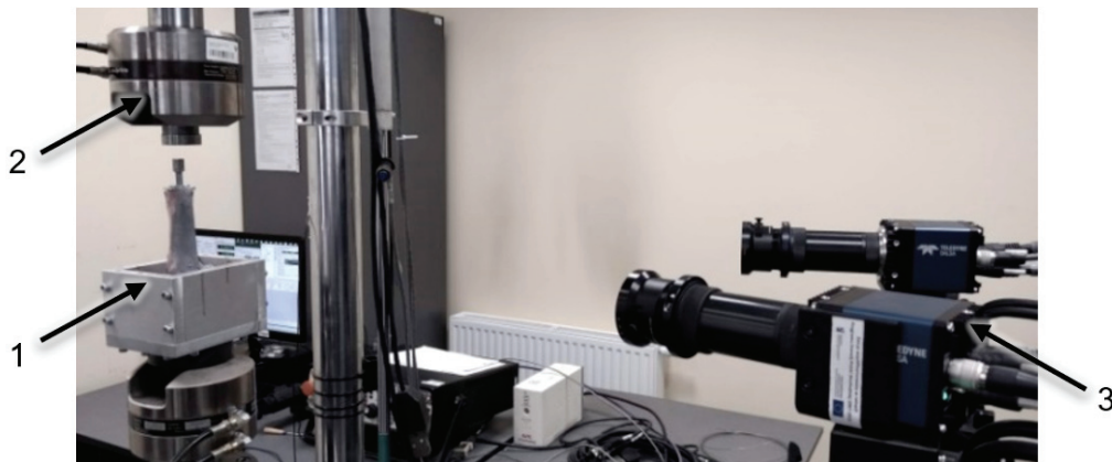
Fig. 7. Stand for testing with the use of a vision system: 1 – aluminium form with the tested sample, 2 – load cell, 3 – ARAMIS 3D 4M vision system
