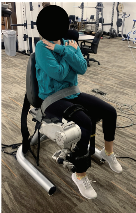
Fig. 2. The Isokinetic Knee Dynamometer prototype used in the current investigation
