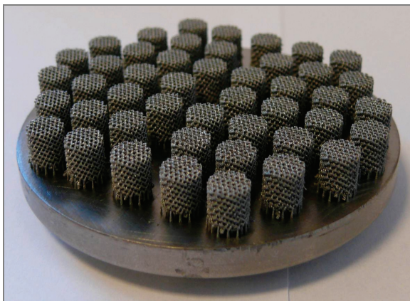
Fig. 1. Scaffolds produced by Selective Laser Melting
