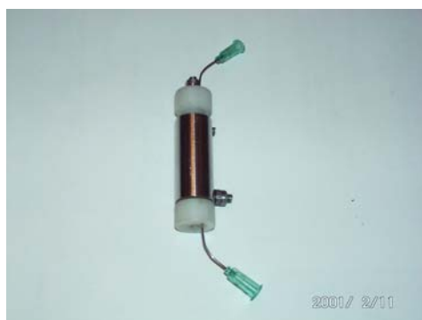
c) electroosmosis chamber for industry
