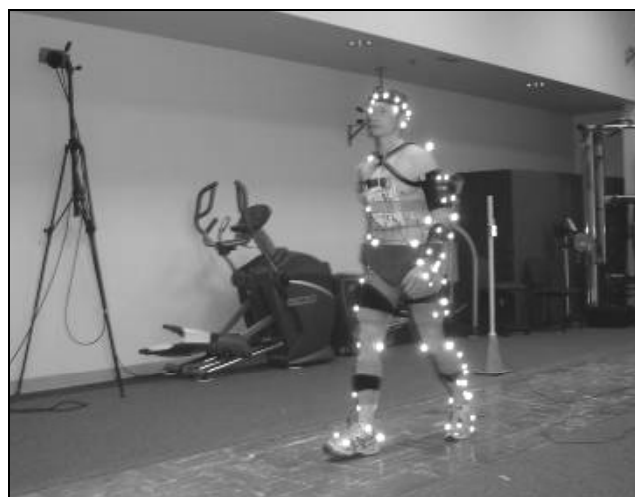
Fig. 7. Gait study with simultaneous recording of stride characteristics (in-shoe footswitches), full body kinematics (passive reflective markers), ground reaction forces (embedded forceplates) and lower extremity muscle activity (surface electrodes)
