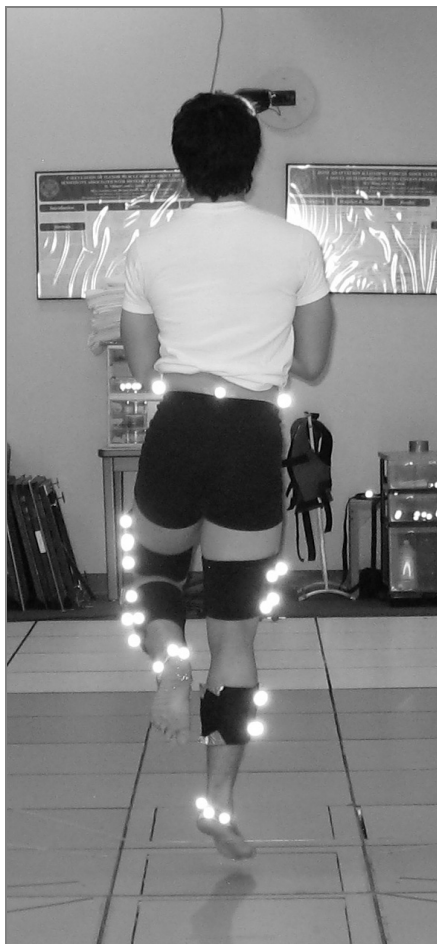
Fig. 5. Subject performing single-legged hopping on a force platform
