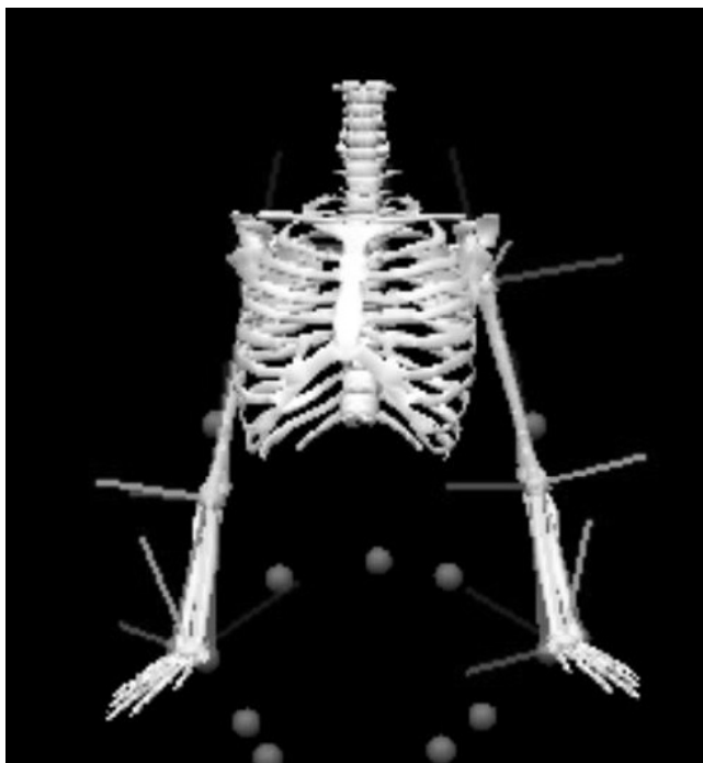
Fig. 2. Model of the upper extremities together with the local reference frames at the wrist, elbow and shoulder
