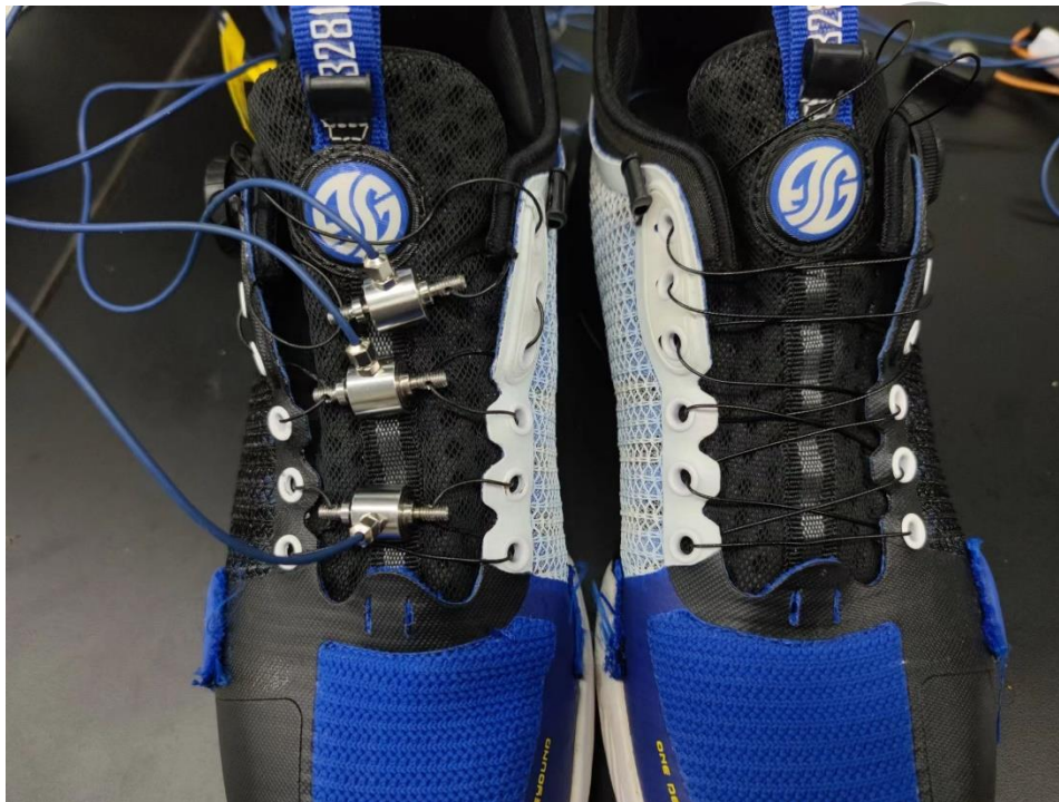
150 151 Figure.2 Three micro force transducers placed in this study
